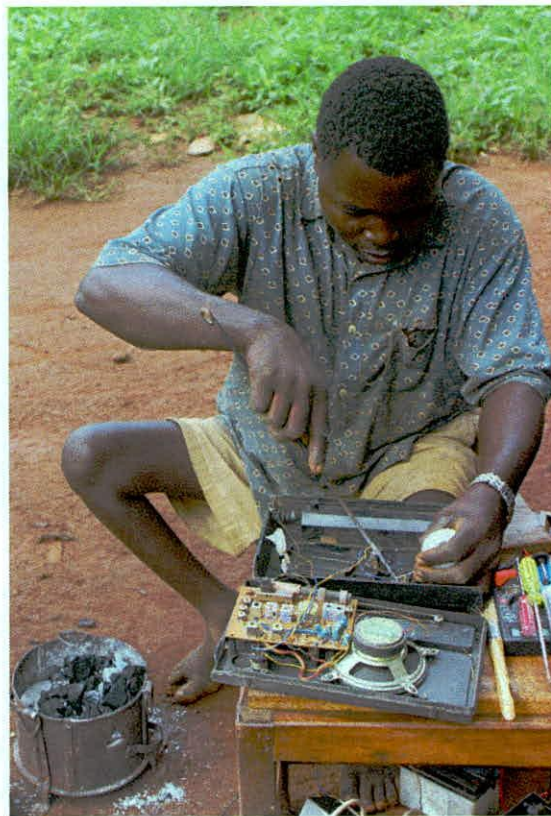
Using charcoal to heat soldering irons
