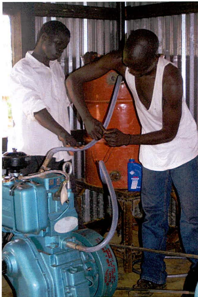
Water cooling system for diesel engine for grinding mill
